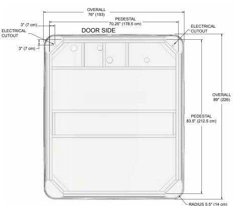
**NOTE: WATKINS WELLNESS** recommends that the **MARTINIQUE** be installed on a minimum 4" (10 cm) thick reinforced concrete pad or structurally sound deck able to support the "dead weight" found in chart on the back page. **WARNING:** The **MARTINIQUE** must not be shimmed in any manner.
