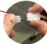
3b Logo Light connector- Push in side clips and pull to remove
