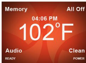
The temperature displayed in the center of the Home screen is the actual temperature of the spa water. If the READY icon is displayed and solid on the control panel, then the actual spa temperature is within 2°F (1°C) of the set temperature. The corner soft button functions are as follows:
