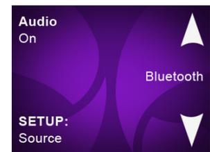
To use the Bluetooth screen, your audio Bluetooth device must be paired with the spa. Audio must be On to use Bluetooth and only one paired Bluetooth device will work at a time.
