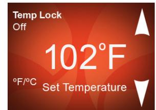
If the set temperature value does not change, check to see whether the TEMP LOCK or SPA LOCK features are on. When either of these features is activated, the temperature control is disabled.
