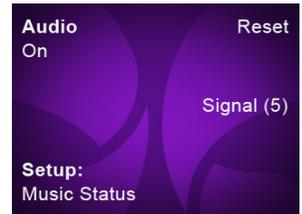
Press the soft button next to **Reset** to disconnect any device using the spa music system so that another paired device may be used. This is also necessary when trying to pair multiple devices because pairing is NOT possible when another device is connected to the music system.
