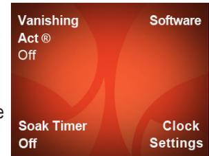
To set Soak Timer for a 30, 45 or 60 minute soak time, press and hold soft button next to **Soak Timer** when timer is Off for several seconds to bring up screen.
