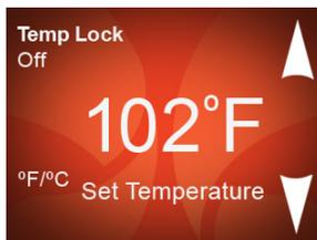
factory. After the spa has been set up and used, the last temperature value set by the user will be stored in memory. If power is disconnected from the spa, it will automatically revert to the last set temperature when power is reapplied.
