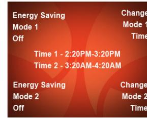
This mode allows you to save energy by shutting off the heater at two predetermine times of the day for up to 6 hours on each setting.
