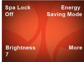
When activated, the Spa Lock feature disables all functions on the control panel. It prevents others from tampering with the jets, lights and temperature settings on your spa. The control panel will not respond to any hard or soft buttons when pushed in Spa Lock mode.
