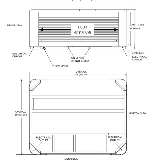
**NOTE: WATKINS WELLNESS** recommends that the Kauai be installed on a minimum 4" (10 cm) thick reinforced concrete pad or structurally sound deck able to support the "dead weight" found in the spa specification chart. **WARNING:** The Kauai must not be shimmed in any manner.
