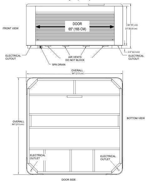
**NOTE:** Watkins Wellness recommends that the Reunion be installed on a minimum 4" (10 cm) thick reinforced concrete pad or structurally sound deck able to support the "dead weight" found in the spa specification chart.
