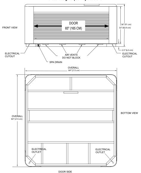
**NOTE:** Watkins Wellness recommends that the Seychelles be installed on a minimum 4" (10 cm) thick reinforced concrete pad or structurally sound deck able to support the "dead weight" found in the spa specification chart.
