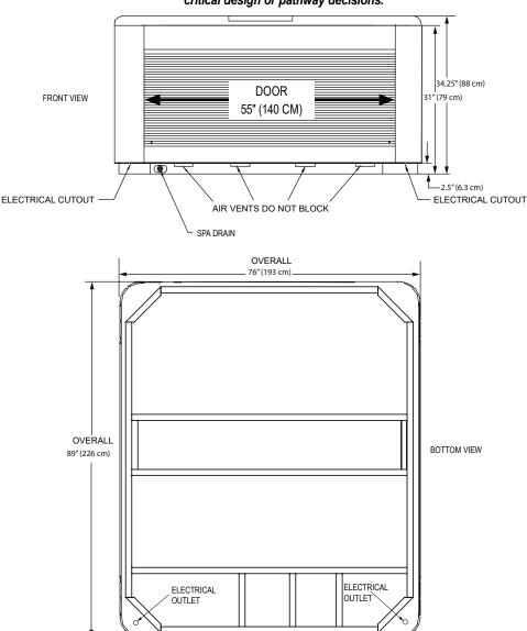
NOTE: WATKINS WELLNESS recommends that the Martinique be installed on a minimum 4" (10 cm) thick reinforced concrete pad or structurally sound deck able to support the "dead weight" found in the spa specification chart
