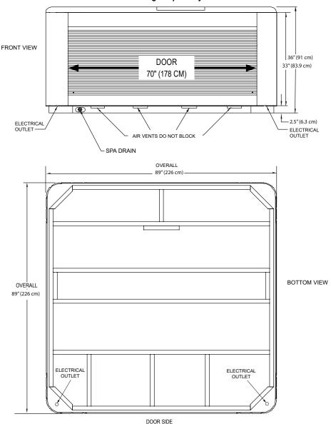
**NOTE: WATKINS WELLNESS** requires that the Makena and Salina be installed on a minimum 4" (10 cm) thick reinforced concrete pad or structurally sound deck able to support the "dead weight" found in the spa specification chart.
