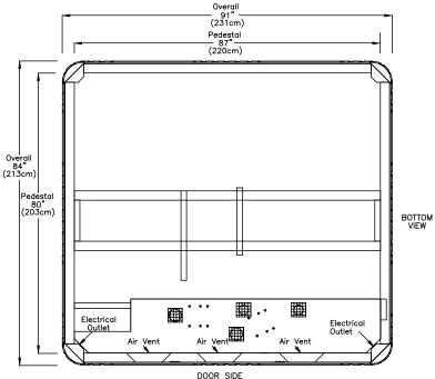
**NOTE:** Watkins Manufacturing Corporation requires that the Moorea be installed on a minimum 4" thick reinforced concrete pad or structurally sound deck able to support the "dead weight" found in the spa specification chart.
