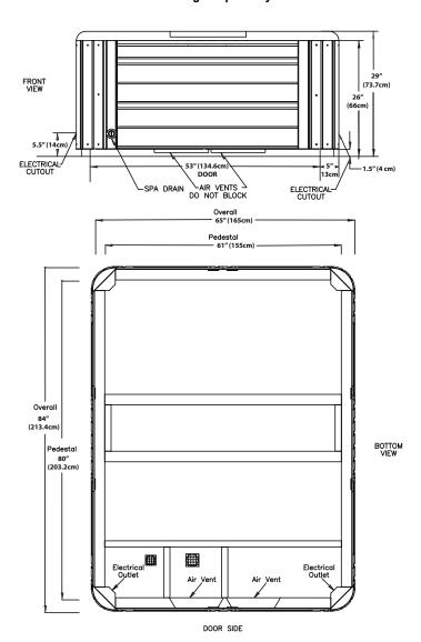
**NOTE:** Watkins Manufacturing Corporation recommends that the Kauai be installed on a minimum 4" thick reinforced concrete pad or structurally sound deck able to support the "dead weight" found in the spa specification chart.
