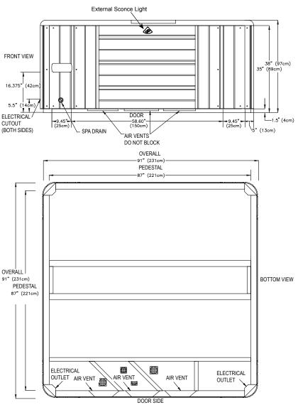
**NOTE:** Watkins Manufacturing Corporation requires that the Elation be installed on a minimum 4" thick reinforced concrete pad or structurally sound deck able to support the "dead weight" found in the spa specification chart.
