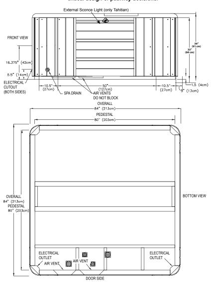
**NOTE:** Watkins Manufacturing Corporation recommends that the Tahitian and Hawaiian be installed on a minimum 4" thick reinforced concrete pad or structurally sound deck able to support the "dead weight" found in the spa specification chart.
