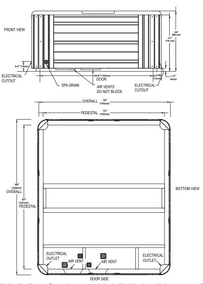
**NOTE:** Watkins Manufacturing Corporation recommends that the Martinique be installed on a minimum 4" thick reinforced concrete pad or structurally sound deck able to support the "dead weight" found in the spa specification chart.
