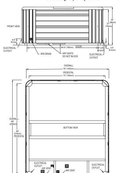
**NOTE:** Watkins Manufacturing Corporation recommends that the Martinique be installed on a minimum 4" thick reinforced concrete pad or structurally sound deck able to support the "dead weight" found in the spa specification chart
