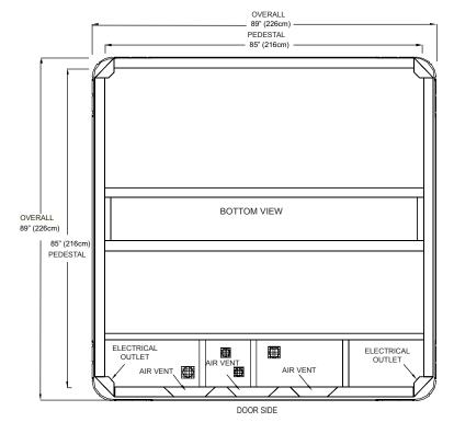
**NOTE:** Watkins Manufacturing Corporation requires that the Makena and Salina be installed on a minimum 4" thick reinforced concrete pad or structurally sound deck able to support the "dead weight" found in the spa specification chart.
