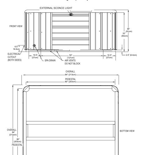
**NOTE:** Watkins Manufacturing Corporation recommends that the Tahitian be installed on a minimum 4" thick reinforced concrete pad or structurally sound deck able to support the "dead weight" found in the spa specification chart.
