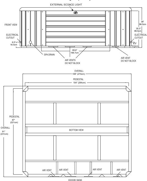
NOTE: Watkins Manufacturing Corporation requires that the Cantabria be installed on a minimum 4" (10 cm) thick reinforced concrete pad or structurally sound deck able to support the "dead weight" found in the spa specification chart
