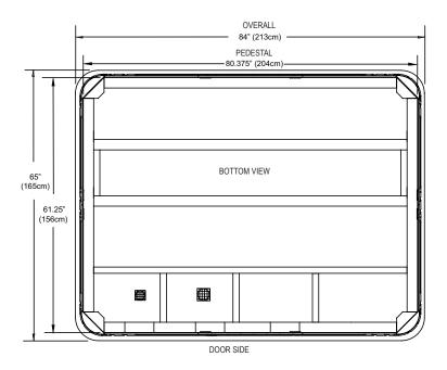
**NOTE:** Watkins Manufacturing Corporation recommends that the Kauai be installed on a minimum 4" thick reinforced concrete pad or structurally sound deck able to support the "dead weight" found in the spa specification chart.
