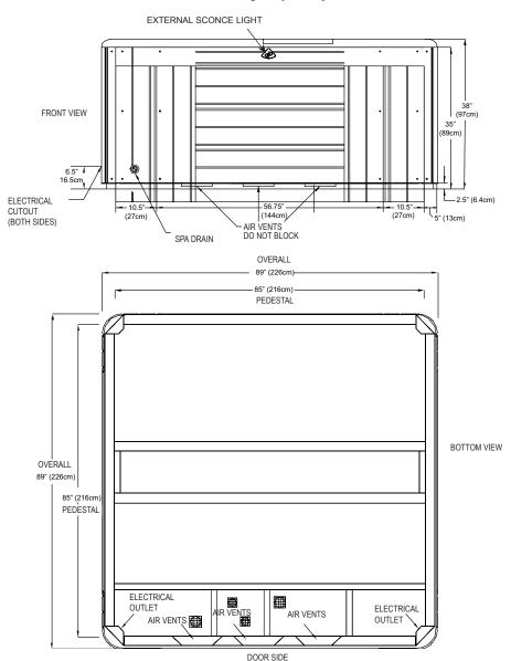
**NOTE:** Watkins Manufacturing Corporation requires that the Geneva and Niagara be installed on a minimum 4" thick reinforced concrete pad or structurally sound deck able to support the "dead weight" found in the spa specification chart.
