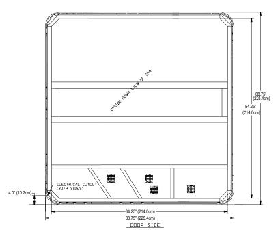
**NOTE:** Watkins Manufacturing Corporation recommends that the Palatino be installed on a minimum 4" (10.2cm) thick reinforced concrete pad or structurally sound deck able to support the "dead weight" found in the spa specification chart.
