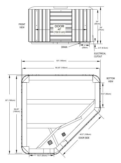
**NOTE:** Watkins Manufacturing Corporation recommends that the **AVENTINE** be installed on a minimum 4" (10 cm) thick reinforced concrete pad or structurally sound deck able to support the "dead weight" found in the spa specification chart.
