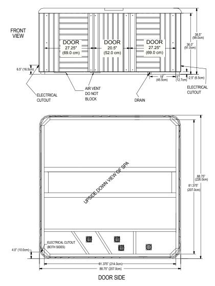
**NOTE:** Watkins Manufacturing Corporation recommends that the **PALATINO** be installed on a minimum 4" (10 cm) thick reinforced concrete pad or structurally sound deck able to support the "dead weight" found in the spa specification chart.
