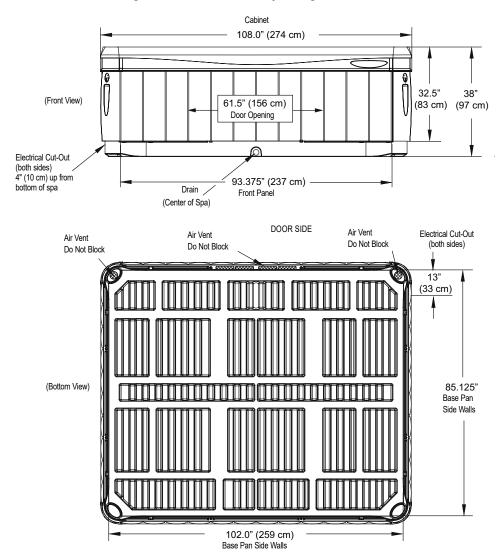
NOTE: WATKINS WELLNESS requires that the CANTABRIA be installed on a minimum 4" (10 cm) thick reinforced concrete pad or structurally sound deck able to support the "dead weight" found in the spa specification chart. WARNING: The CANTABRIA must not be shimmed in any manner.
