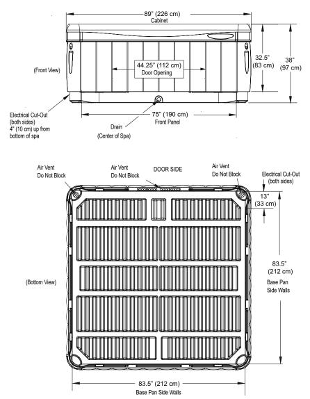
**NOTE: WATKINS WELLNESS** requires that the **GENEVA** and **NIAGARA** be installed on a minimum 4" (10 cm) thick reinforced concrete pad or structurally sound deck able to support the "dead weight" found in the spa specification chart.
