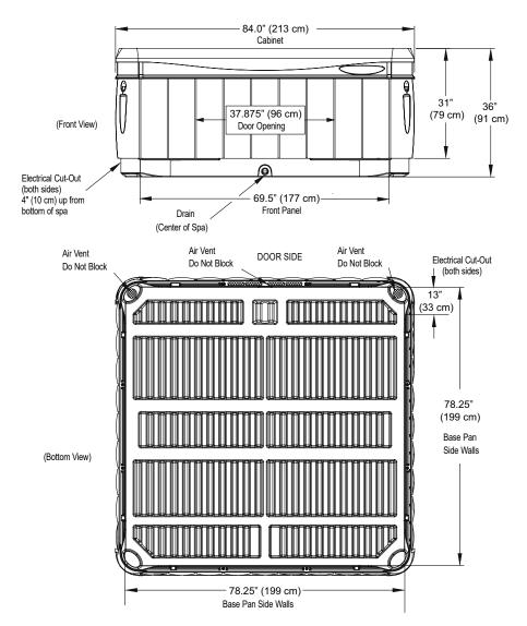
**NOTE: WATKINS WELLNESS** recommends that the **TAHITIAN** and **FLORENCE** be installed on a minimum 4" (10 cm) thick reinforced concrete pad or structurally sound deck able to support the "dead weight" found in the spa specification chart.
