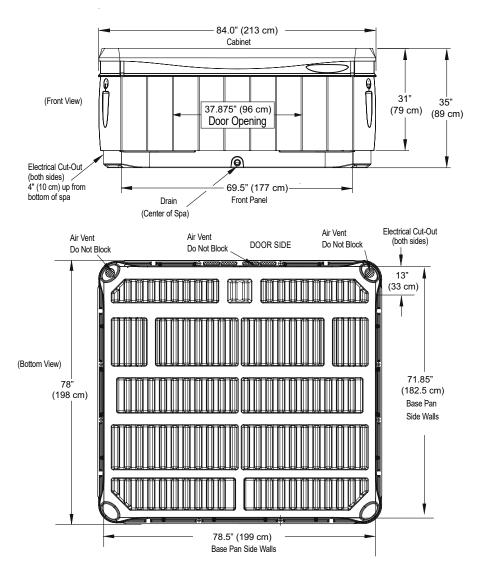
NOTE: WATKINS WELLNESS requires that the **PROVENCE** be installed on a minimum 4" (10 cm) thick reinforced concrete pad or structurally sound deck able to support the "dead weight" found in the spa specification chart.
