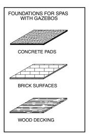
As a homeowner, it is your responsibility to provide a suitable, level foundation for your spa. Keep in mind that most delivery crews are not equipped to level and prepare spa sites. Shimming or point leveling is NOT supported or recommended by the manufacturer.
