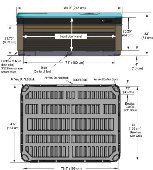
**NOTE: WATKINS WELLNESS** recommends that the **RAVELLO** be installed on a minimum 4" (10 cm) thick reinforced concrete pad or structurally sound deck able to support the "dead weight" found in the spa specification chart. **WARNING:** The **RAVELLO** must not be shimmed in any manner.
