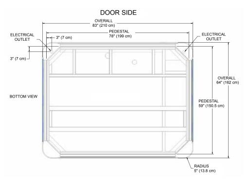
**NOTE: WATKINS WELLNESS** recommends that the **CELIO** be installed on a minimum 4" (10 cm) thick reinforced concrete pad or structurally sound deck able to support the "dead weight" found in the spa specification chart. **IMPORTANT:** The **CELIO** must not be shimmed in any manner.
