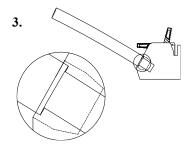
Insert wire fully into Terminal Block
